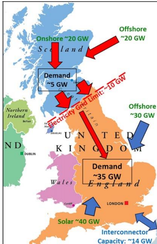
Figure 3.1: UK electricity generation capacity & average demand 2030 with grid limits (pers. comm. J. Briggs, 2024)
