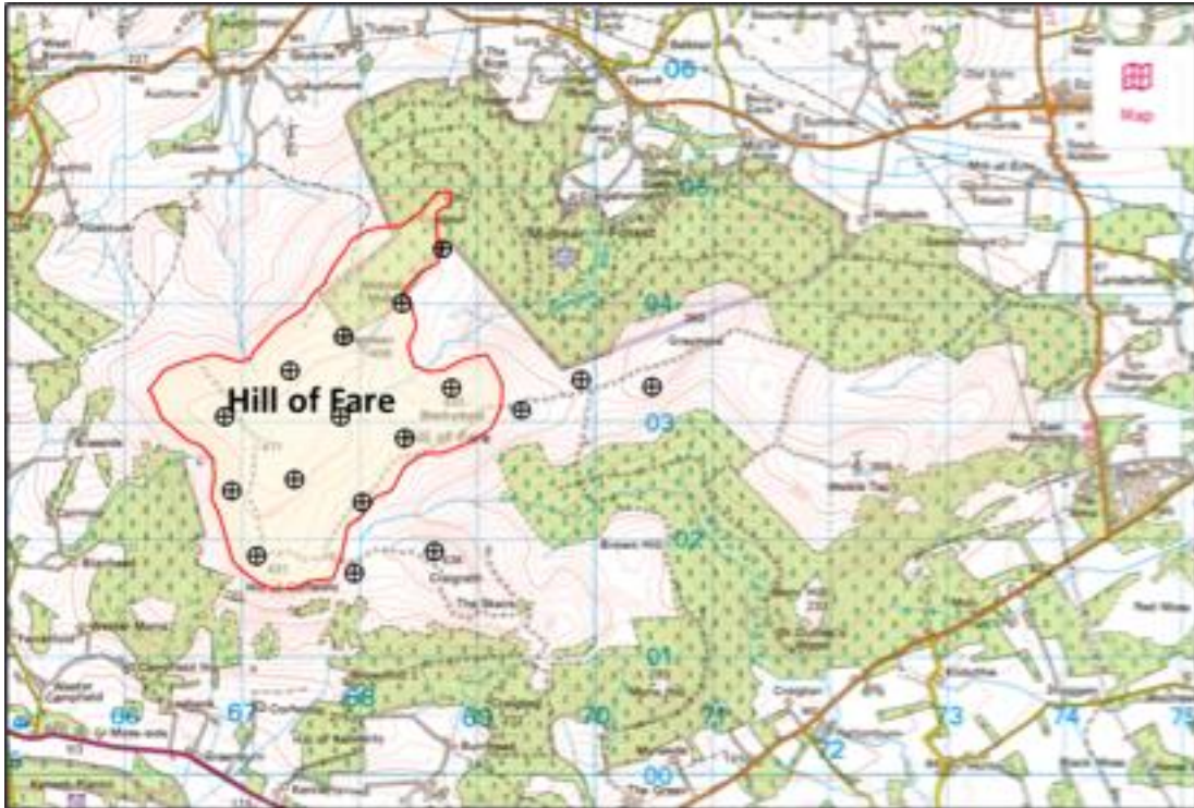
Figure 5.1: Ordnance Survey map with area above 400m marked by red line and proposed 16 turbines showing their prominent position on the highest areas of the Hill of Fare ridge.
